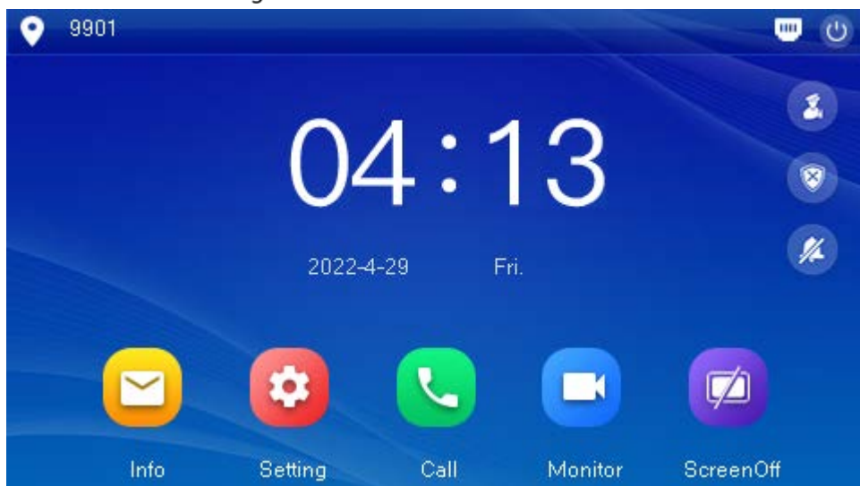
Figure 4-7 VTH main interface
