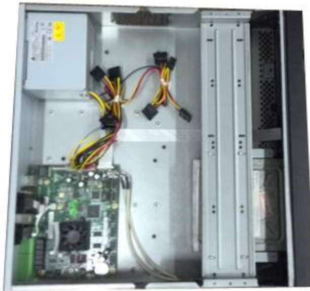
Figure 3-45 Put bracket back
