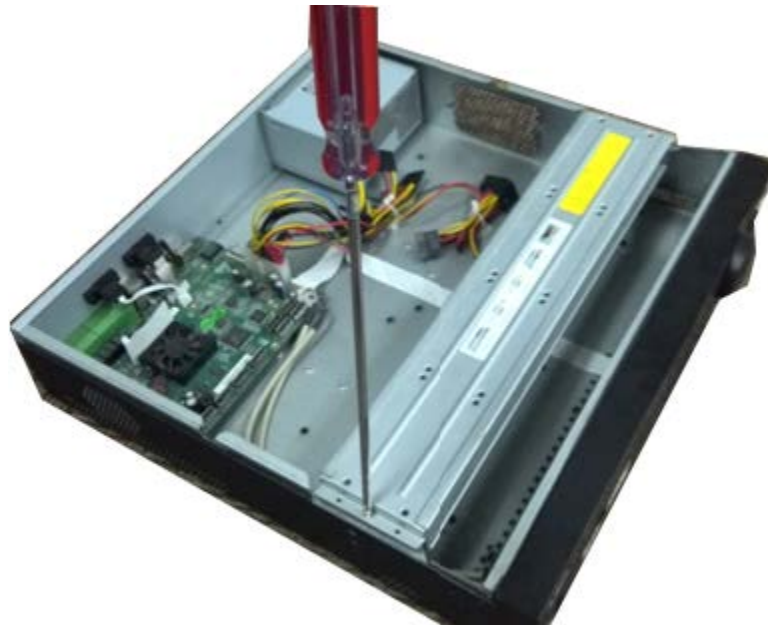
Figure 3-37 Open the top cover
