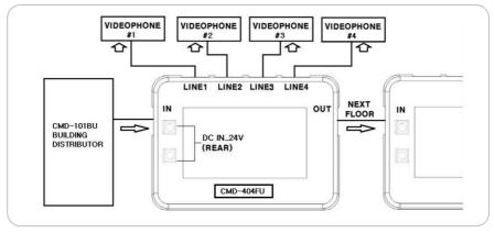
• CCTV / LOBBY → Building distributor(CMD-101BU) → CMD-404FU(D)(1<sup>ST</sup> FLOOR) → CMD-404FU(D)(1<sup>ST</sup> FLOOR) → ... → MODUME VIDEO PHONE
