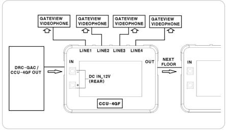
DRC-GAC(LOBBY) CCU-4GF(1<sup>st</sup> FLOOR) → CCU-4GF(2<sup>ND</sup> FLOOR) → ... →
